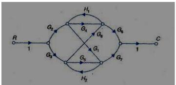
Using block diagram reduction technique find the closed loop transfer Function of the system whose block diagram is given in figure below.
